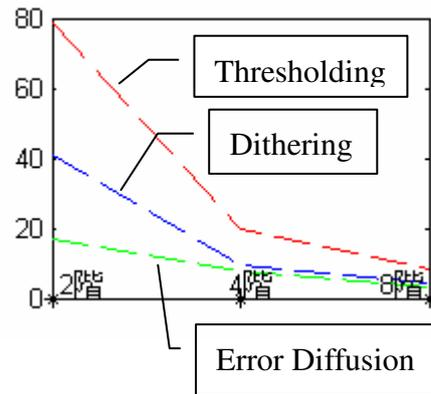
Figure 7 The root-mean-square error evaluated after a 3x3 average filtering.
