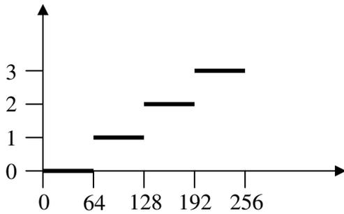
Figure 1 The mapping function of a 4-grayscale uniform thresholding.
