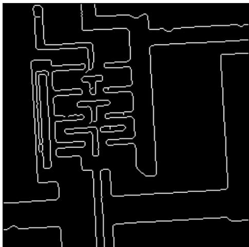
Figure 10(b) The edge image produced by the Canny's edge detection algorithm.
