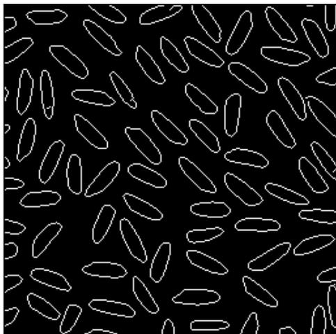
Figure 11(b) The edge image produced by the Canny's edge detection algorithm.
