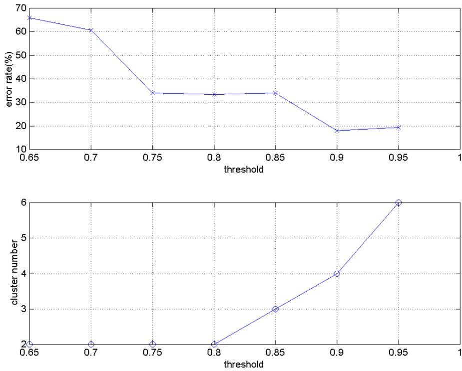
Fig. 10 The error rate and cluster number of ART at different threshold values
