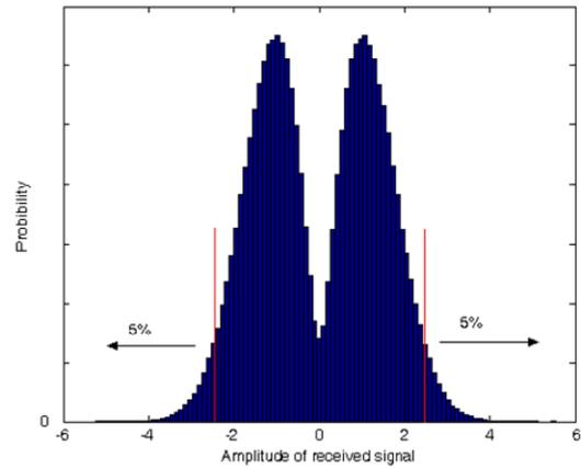
Fig. 6 The chosen quantization range
