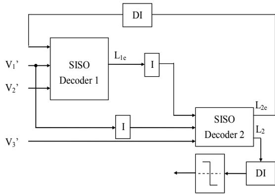
Fig. 3 Turbo code decoder
