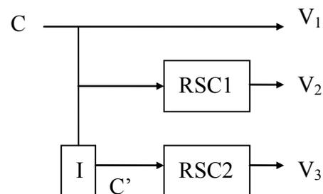
Fig. 2 The turbo code encoder
