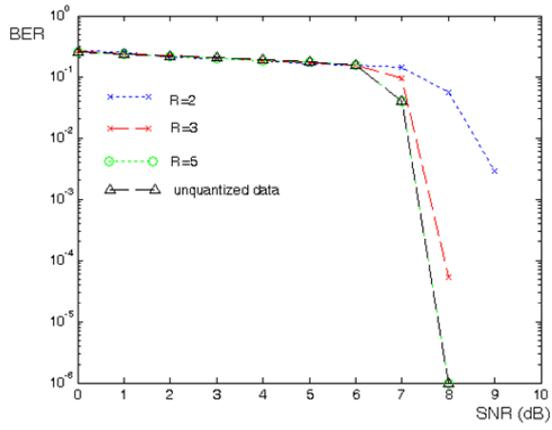
Fig. 9 Effect of quantization bits on turbo code performance under an AWGN channel
