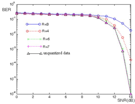
Fig. 10 Effect of quantization bits on turbo code performance under Rayleigh fading channel
