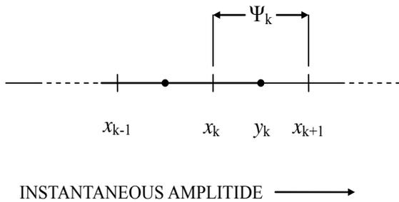
Fig4. Quantization of received signal
