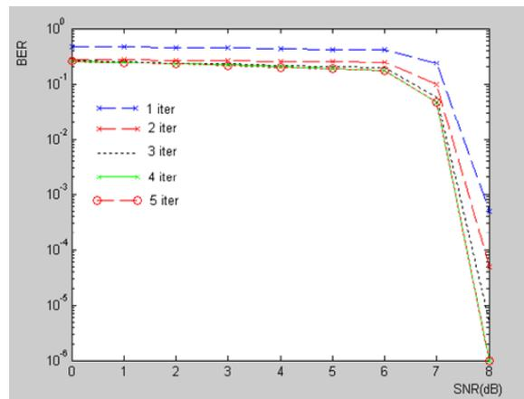
Fig. 7 Effect of iterations on turbo code performance using the Bi-SOVA under AWGN channel
