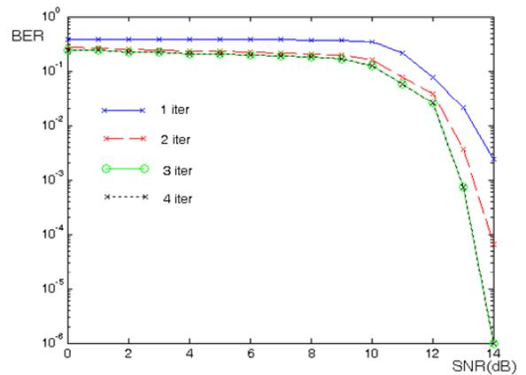
Fig. 8 Effect of iterations on turbo code performance using the Bi-SOVA under Rayleigh fading channel
